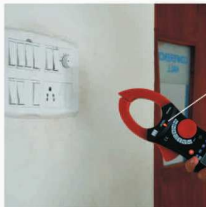
NCV Detect Voltage at Electrical outlet Powercord Terminal strip
